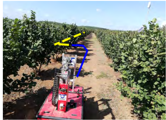
Fig. 1: A farming robot navigating a hazelnut orchard environment. The field traversing route is represented by the blue solid and the yellow dotted (the part of the route on the other row) lines.
