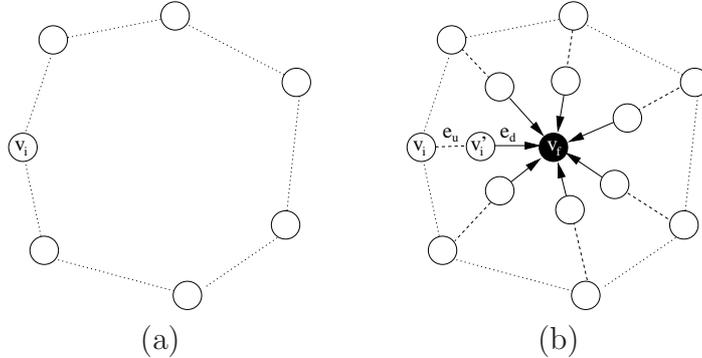
Figure 5: The *triangulation* operation: (a) A face  $f$  with more than three vertices. (b) The same face after vertex  $v_f$  has been inserted and joined to the boundary of  $f$  with paths of length 2.
